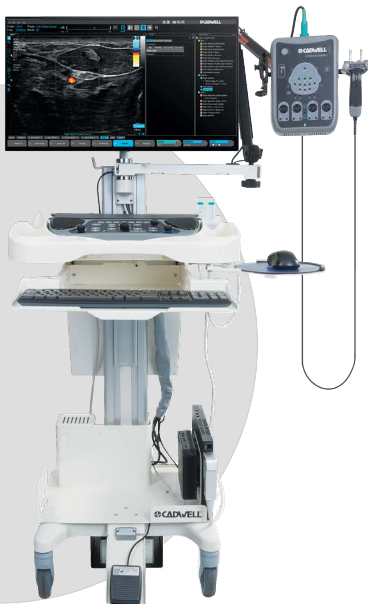
Sierra Summit® 12-channel amplifier and Sierra NMUS1® Ultrasound configuration, with High-Performance Mini PC
