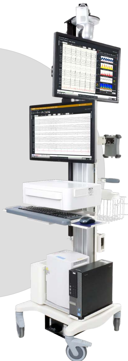
Arc Apollo+ Configuration with Small Form Factor PC and dual-stacked monitors
