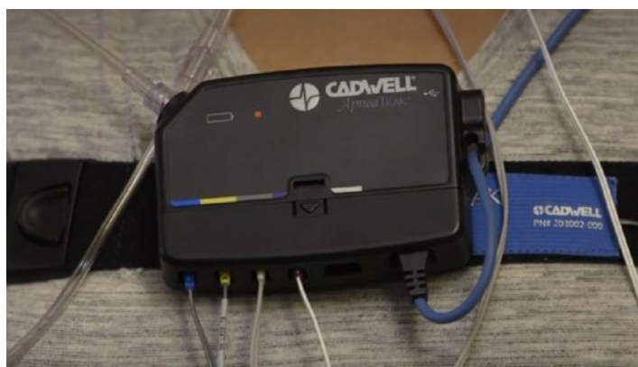
Recessed connections are protected, and elevated from the patient's body to improve comfort and reduce overall size.
